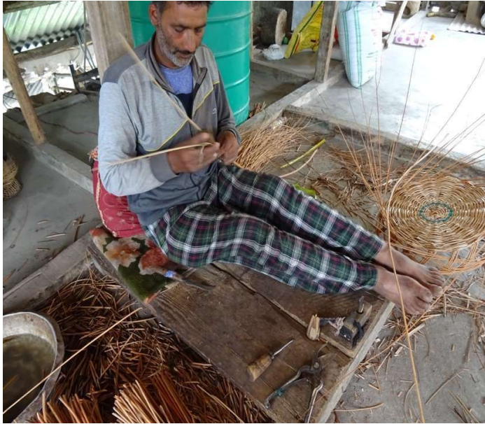
Fig. 1 Splitting of Wicker withies to desirable Size
